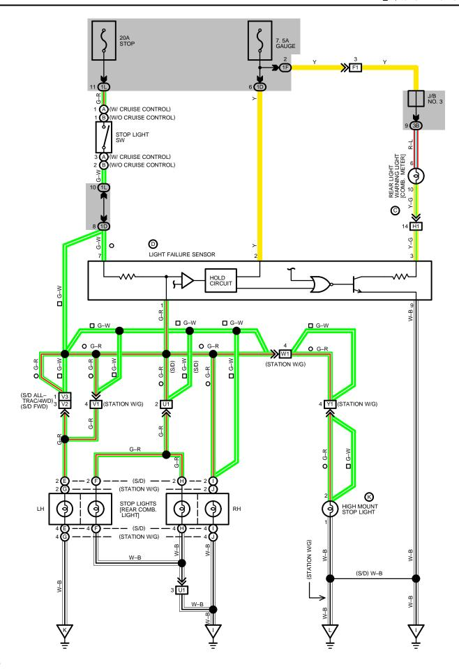
CURRENT IS APPLIED AT ALL TIMES THROUGH A STOP FUSE TO TERMINAL 1 OF THE STOP LIGHT SW.
